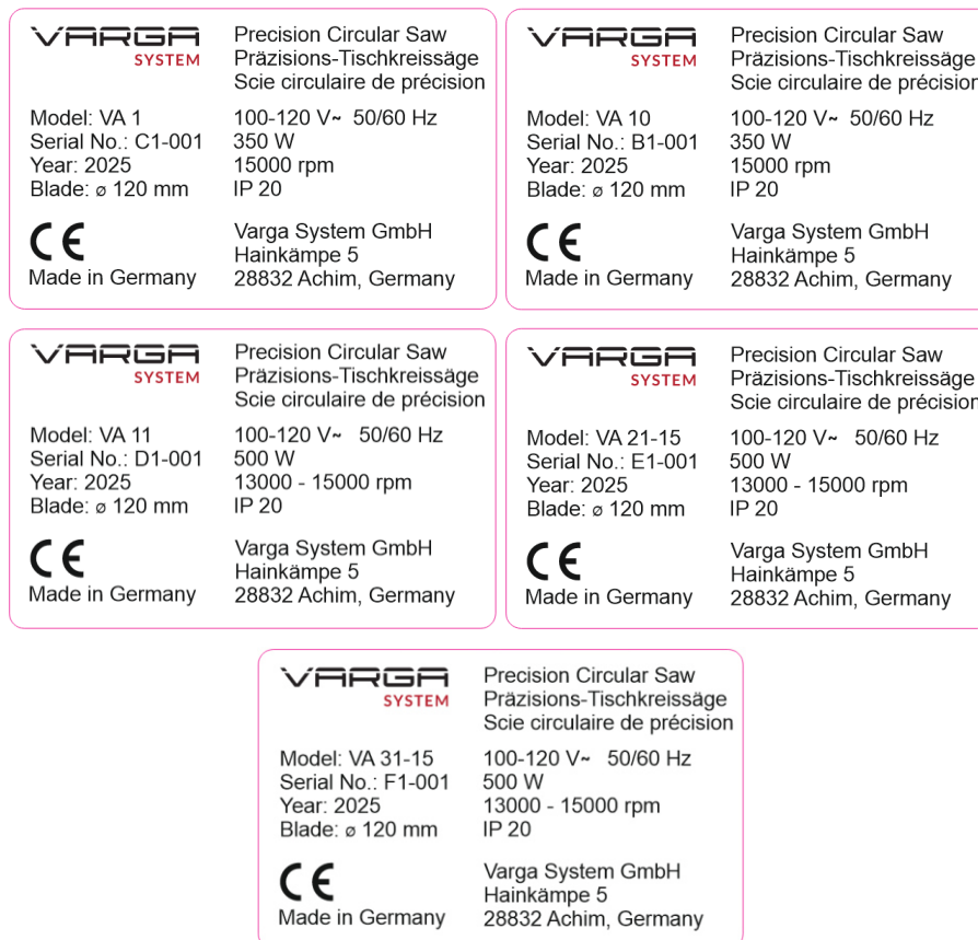
Figure 4 Machine type plates 100-120 V~ mains voltage
