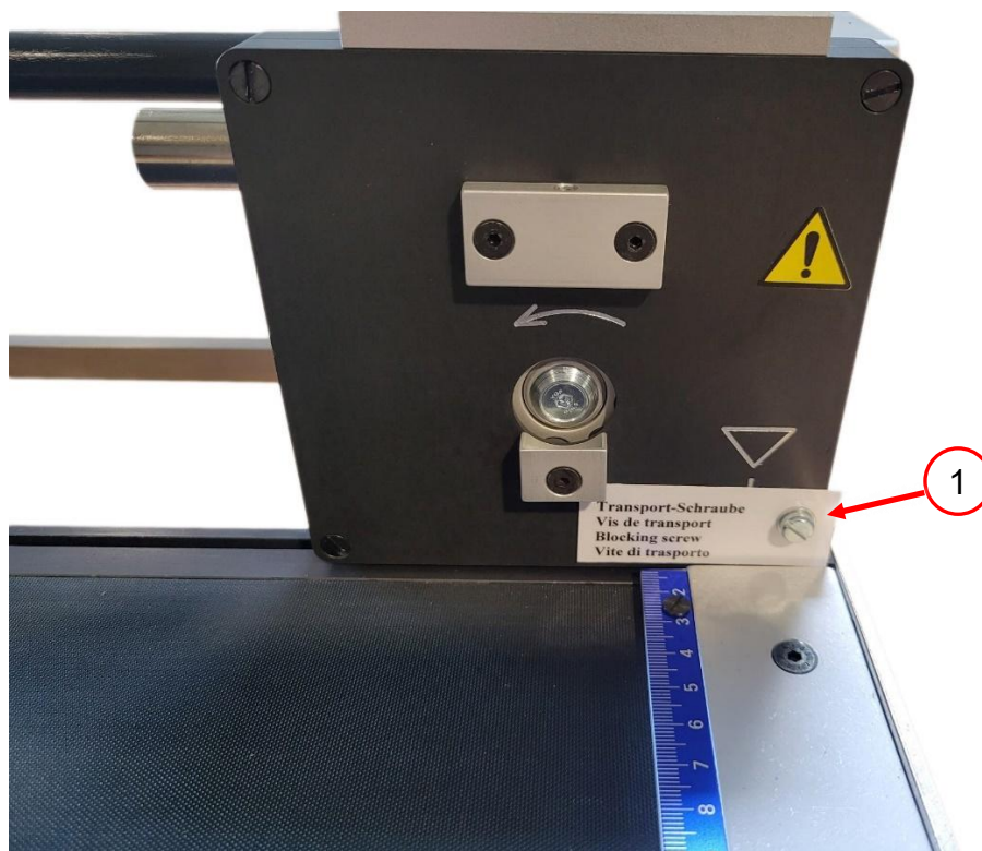
Figure 42 Remove transport screw and plastic ring VARGA VA 1
